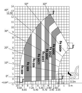
Machine on lowered stabilisers with forks Metric
