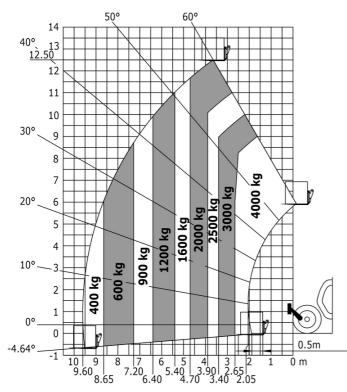
Machine on lowered stabilisers with forks Metric
