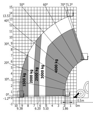
Machine on lowered stabilisers with forks Imperial
