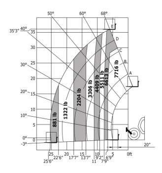
Machine on lowered stabilisers with forks Metric
