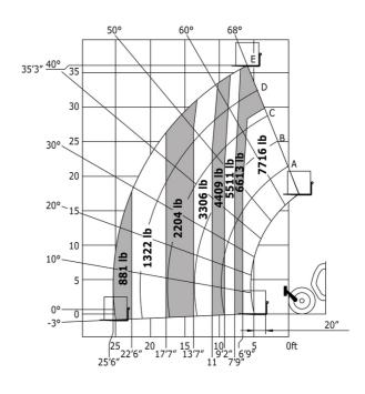
Machine on lowered stabilisers with forks Metric
