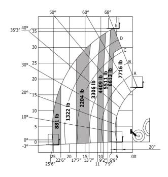
Machine on lowered stabilisers with forks Metric
