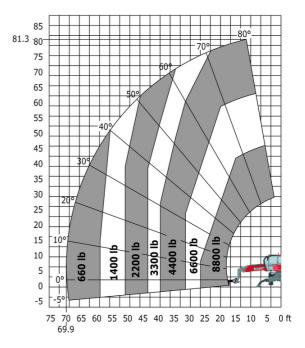
Machine on lowered stabilisers with 1500 kg jib with winch Machine on lowered stabilisers with hook 5000 kg (Imperial)
