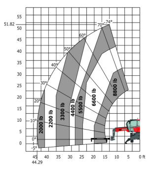
Machine on lowered stabilisers with 1500 kg jib with winch Machine on lowered stabilisers with hook 5000 kg (Imperial)
